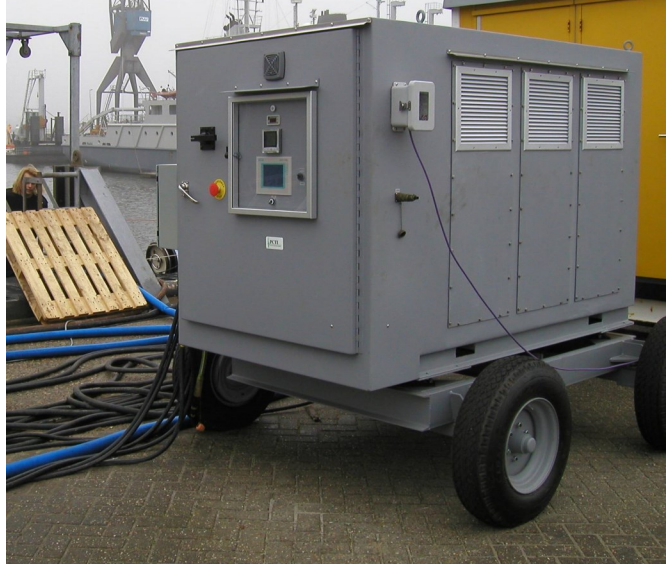
Dutch Navy Battery Charger and Discharger for Submarine Batteries Dual Input: 440V/50Hz, 480V, 60Hz. Output: 400ADC & 800ADC 350-650VDC, 520KW & 260KW
